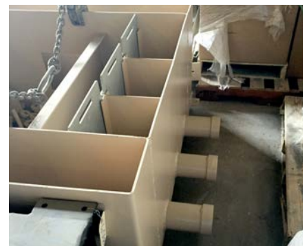
Flow Distribution Chamber
