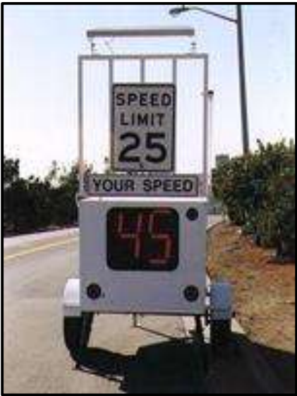
Radar Trailer. Source: City of Pacifica.
