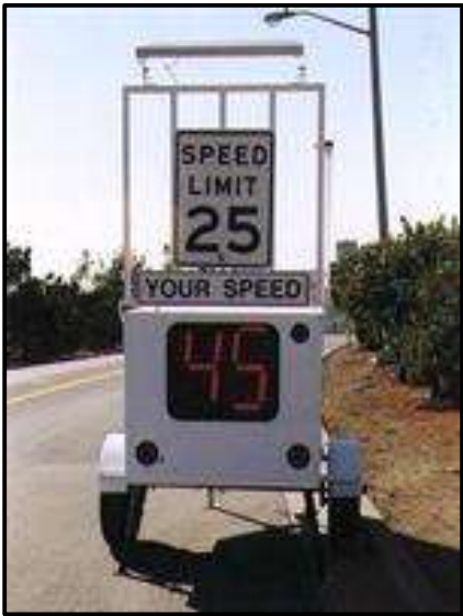
Radar Trailer. Source: City of Pacifica.
