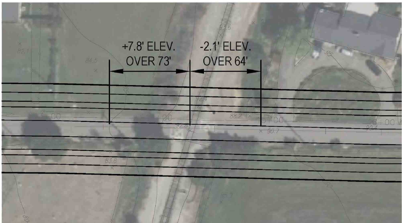
Figure 9. Watson Lane Reconfiguration (Alternative 4); Existing Elevation Change at Railroad Tracks
