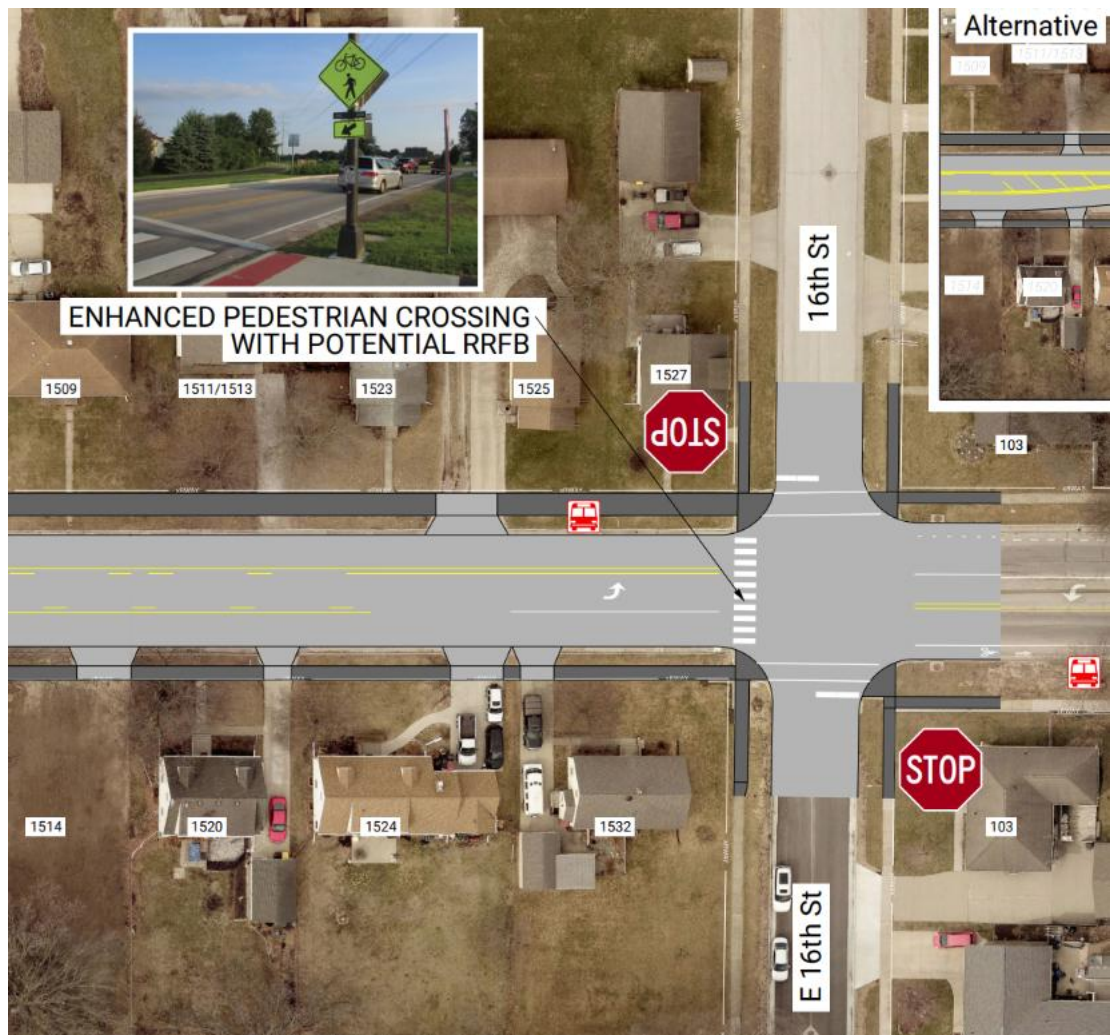
Figure 14: Conceptual Design Option with RRFB Crossing at 16 th Street
