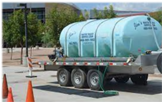
Figure 8.8: Potable Water Tank Trailer
