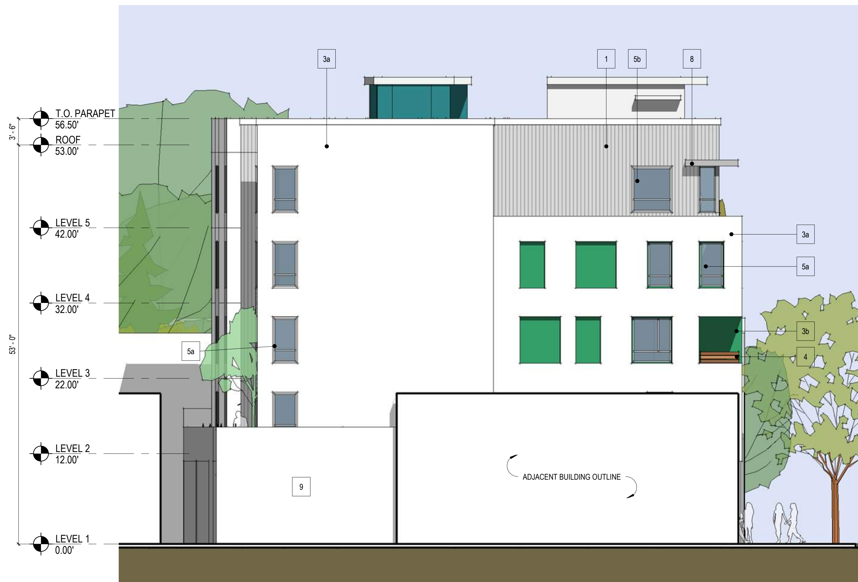
2 Site A South-East Elevation 1/8" = 1'-0"
