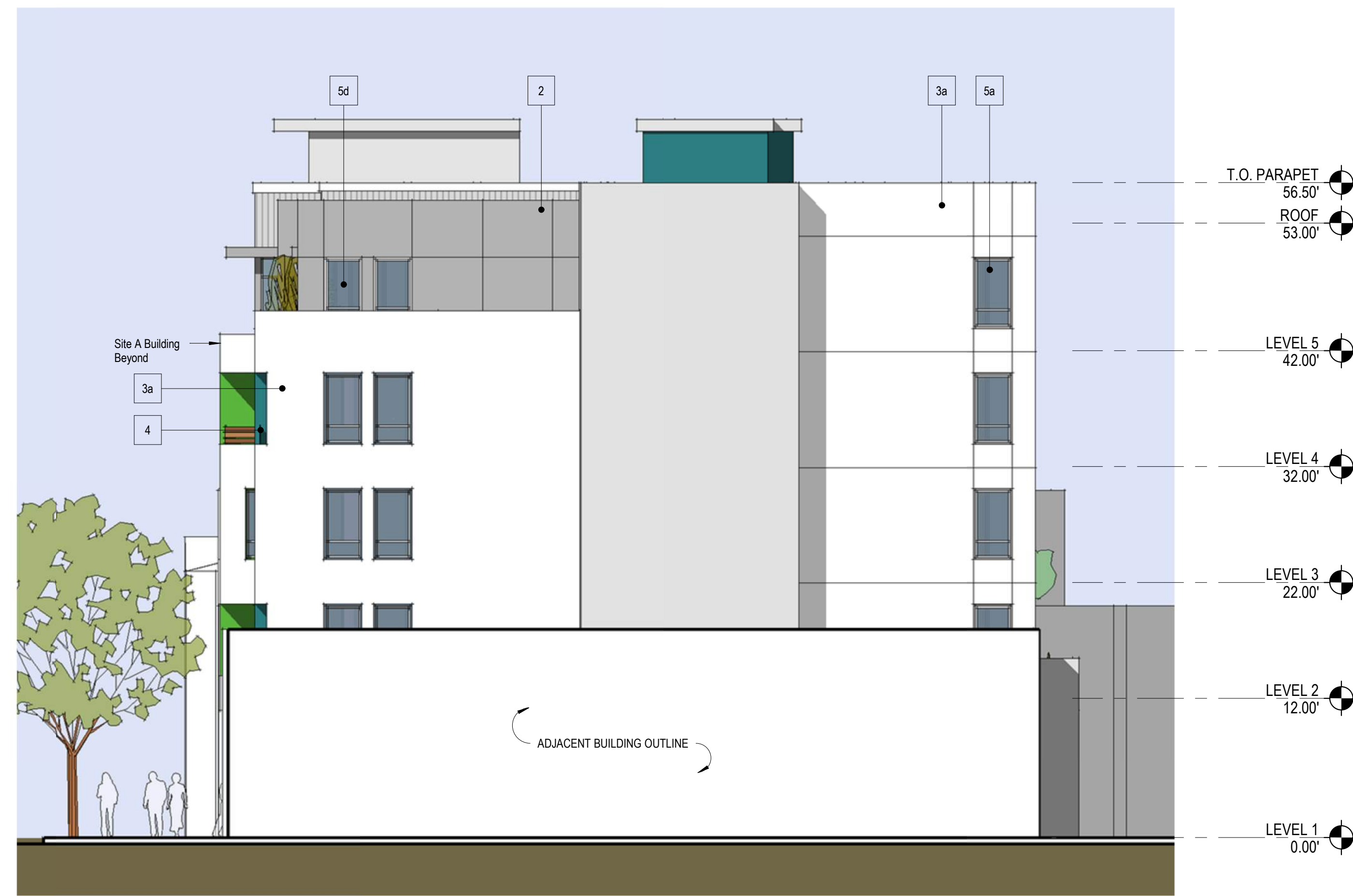
3 Site B North-West Elevation 1/8" = 1'-0"
