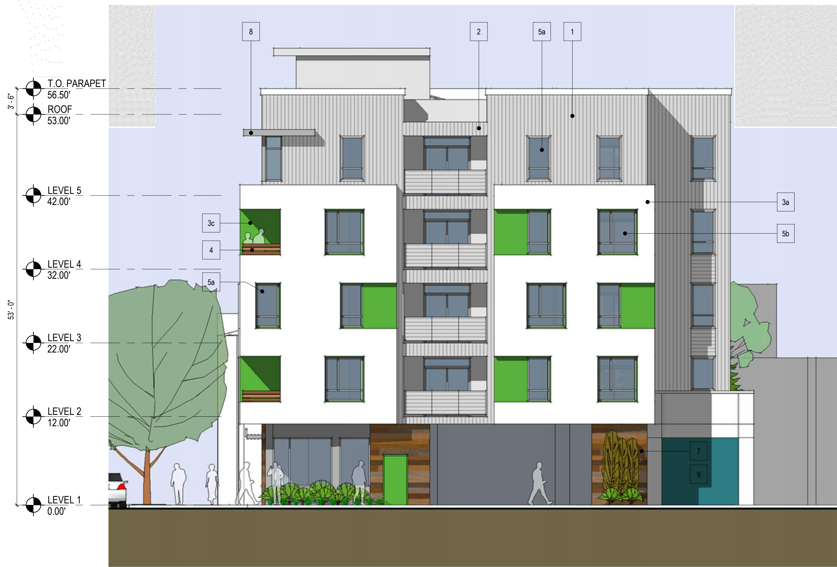
3 Site A Hill Street Elevation 1/8" = 1'-0"
