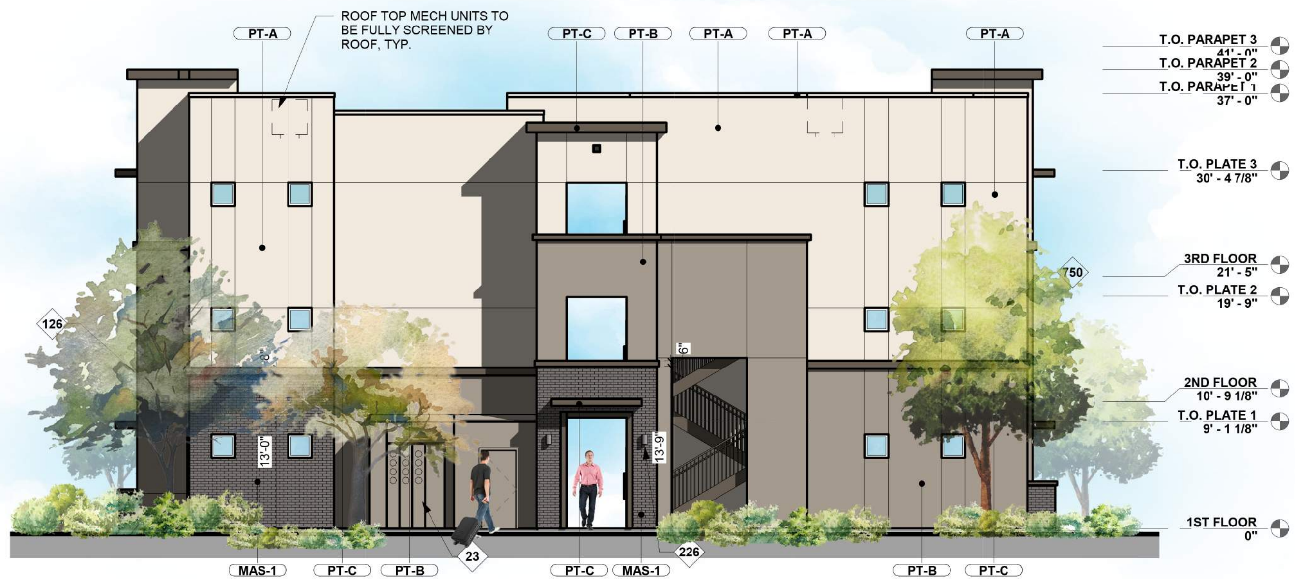
3 ELEVATION BLDG 1 SIDE - RIGHT STREET 1/8" = 1'-0"
