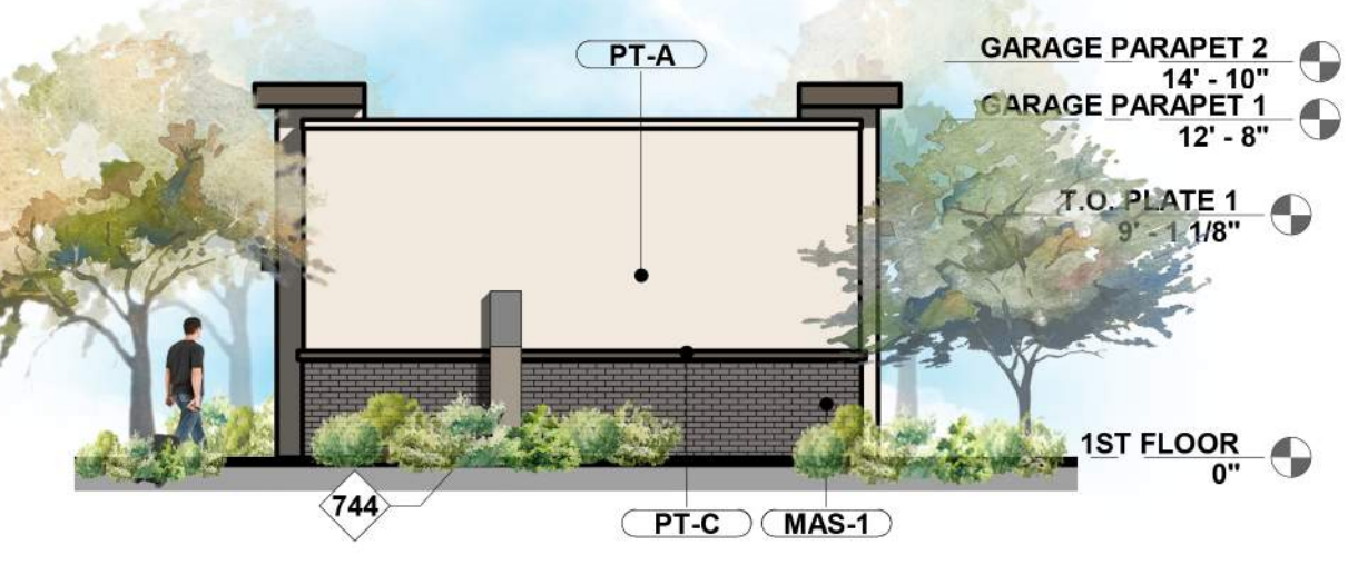
4 ELEVATION GARAGE END 1/8" = 1'-0"
