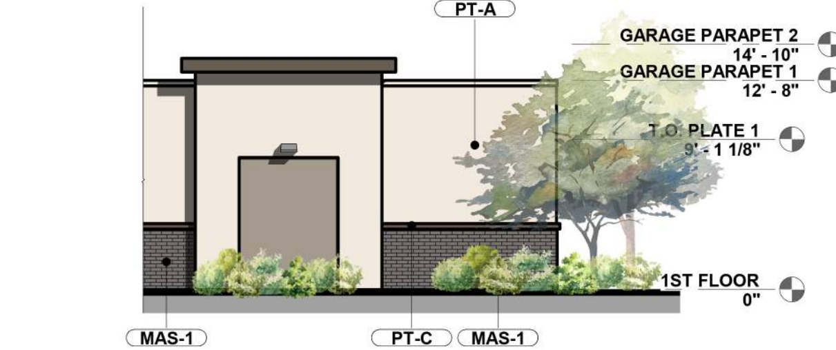
2.1 ELEVATION GARAGE REAR - INT. BLDG 1/8" = 1'-0"
