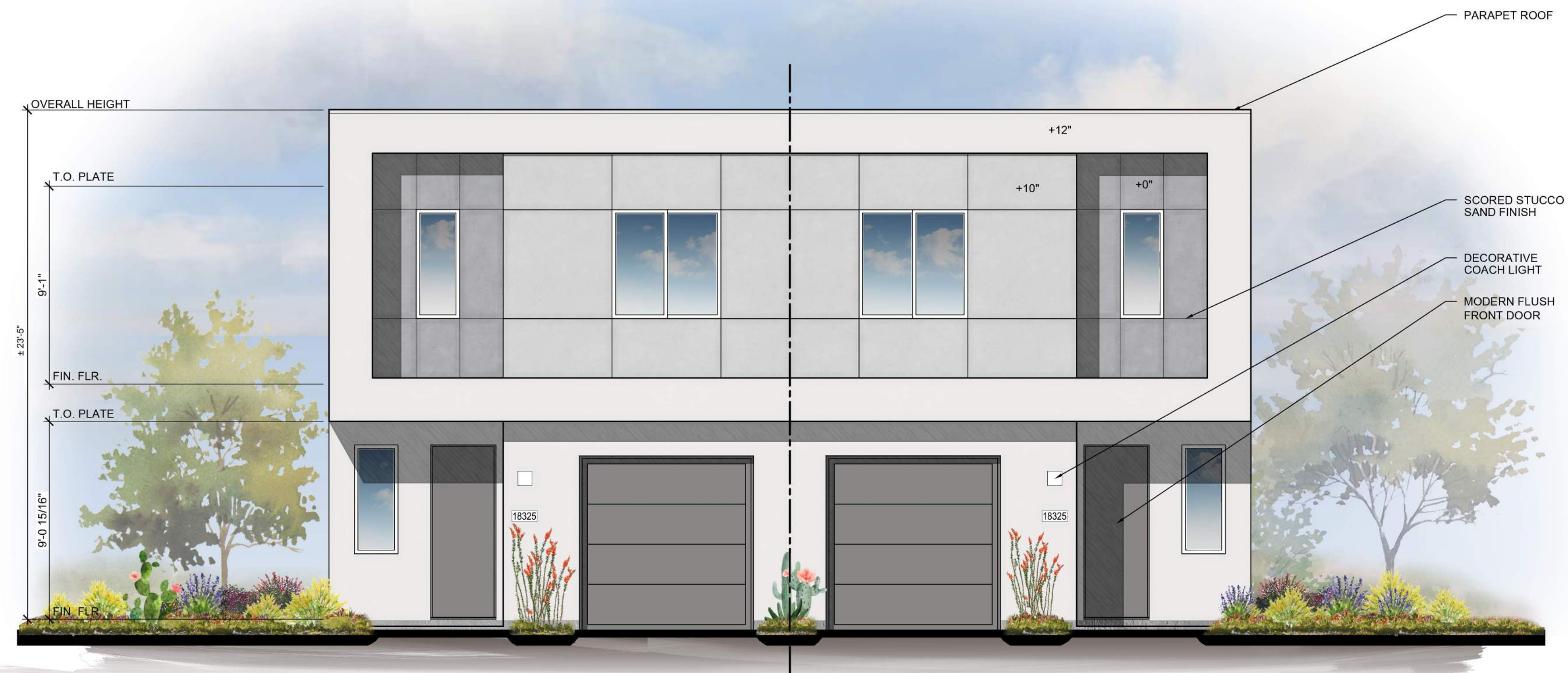
FRONT ELEVATION ELEVATION E-E 1/4" = 1'-0"
