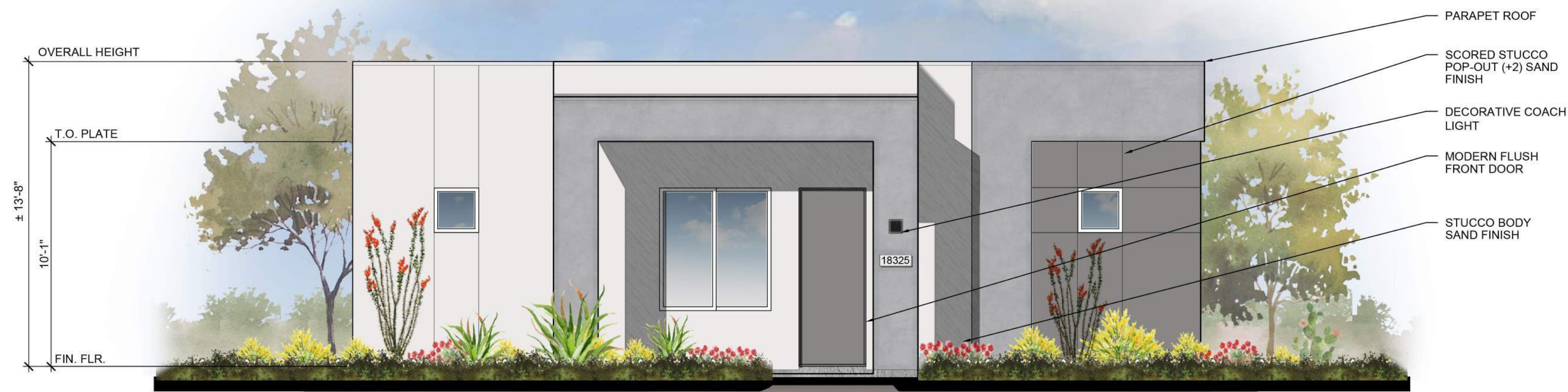
FRONT ELEVATION ELEVATION C 1/4" = 1'-0"
