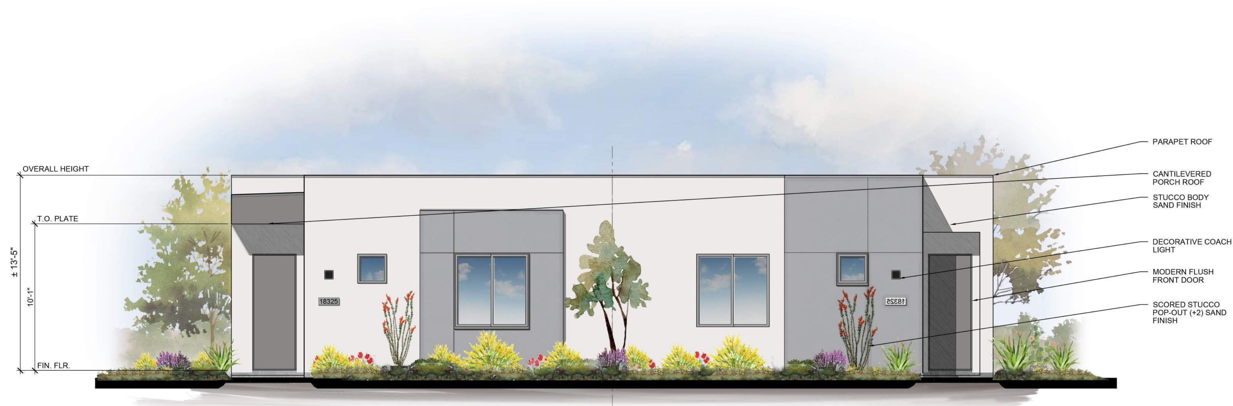
FRONT ELEVATION ELEVATION A-B 1/4" = 1'-0"
