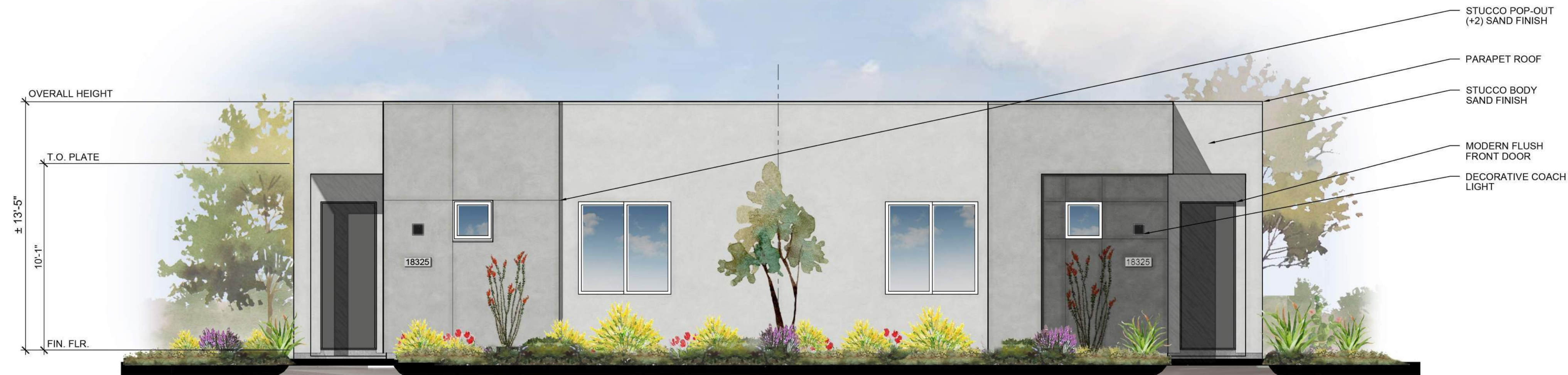
FRONT ELEVATION ELEVATION B-C 1/4" = 1'-0"
