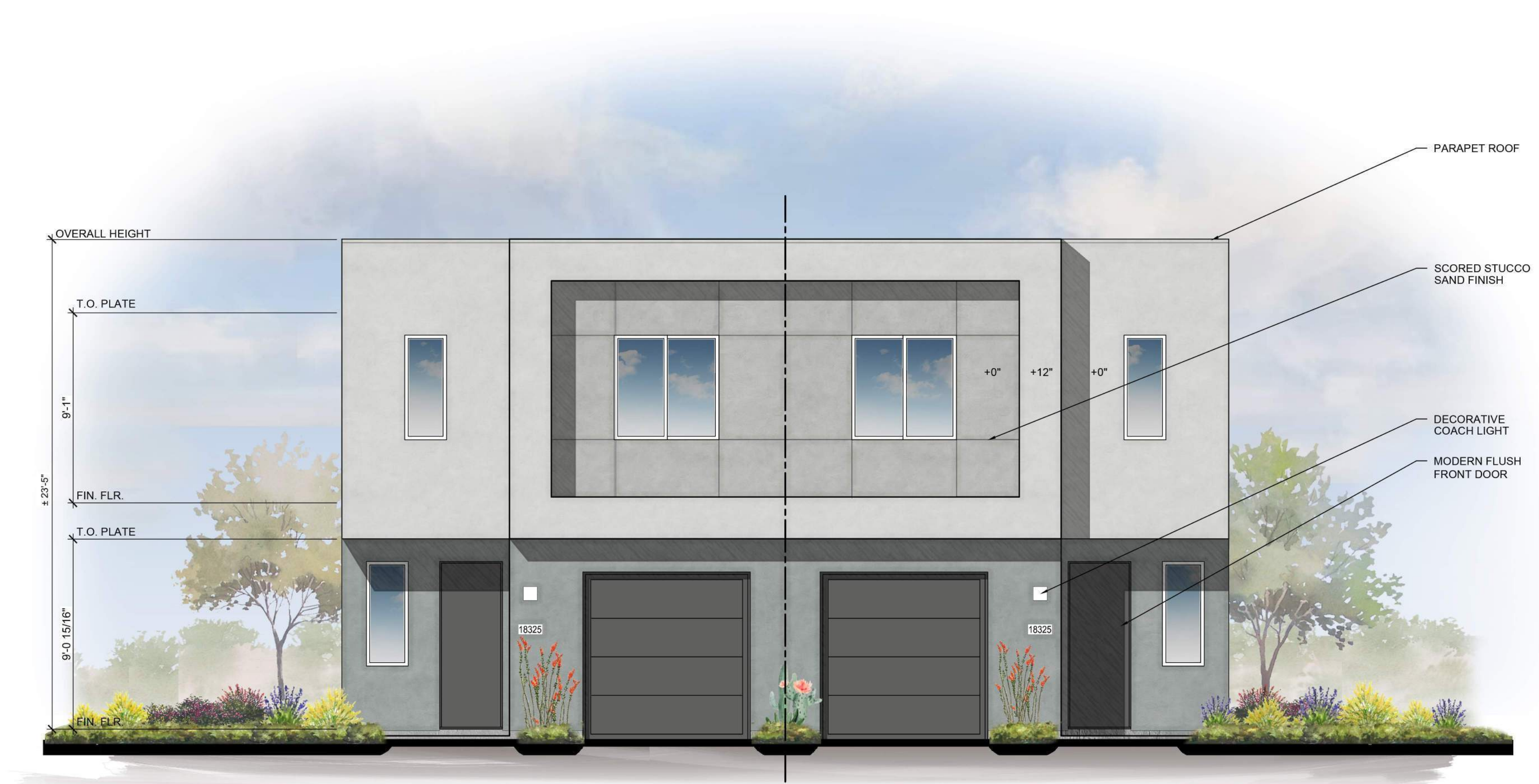
FRONT ELEVATION ELEVATION C-C 1/4" = 1'-0"
