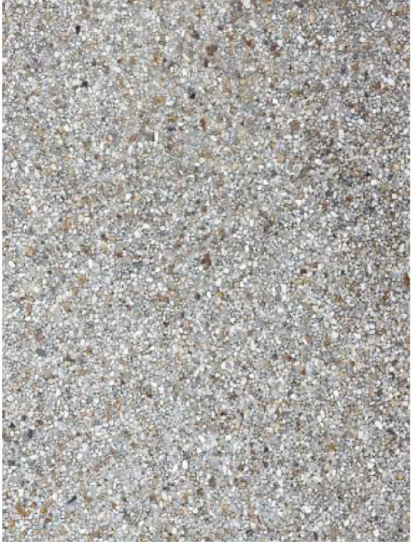
CONC-2 Tilt-up Concrete with Sandblasted Texture (Stained in select BOH areas)
