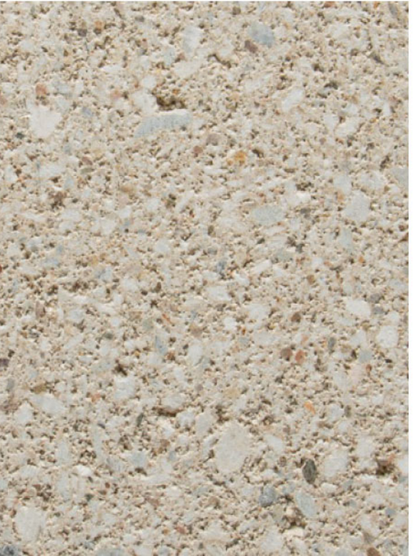
CMU-4 Echelon Trendstone - Mission White - Stacked Bond (Feature Wall)
