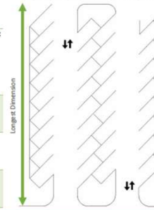
Figure 47. Longest Dimension of Parking Area
