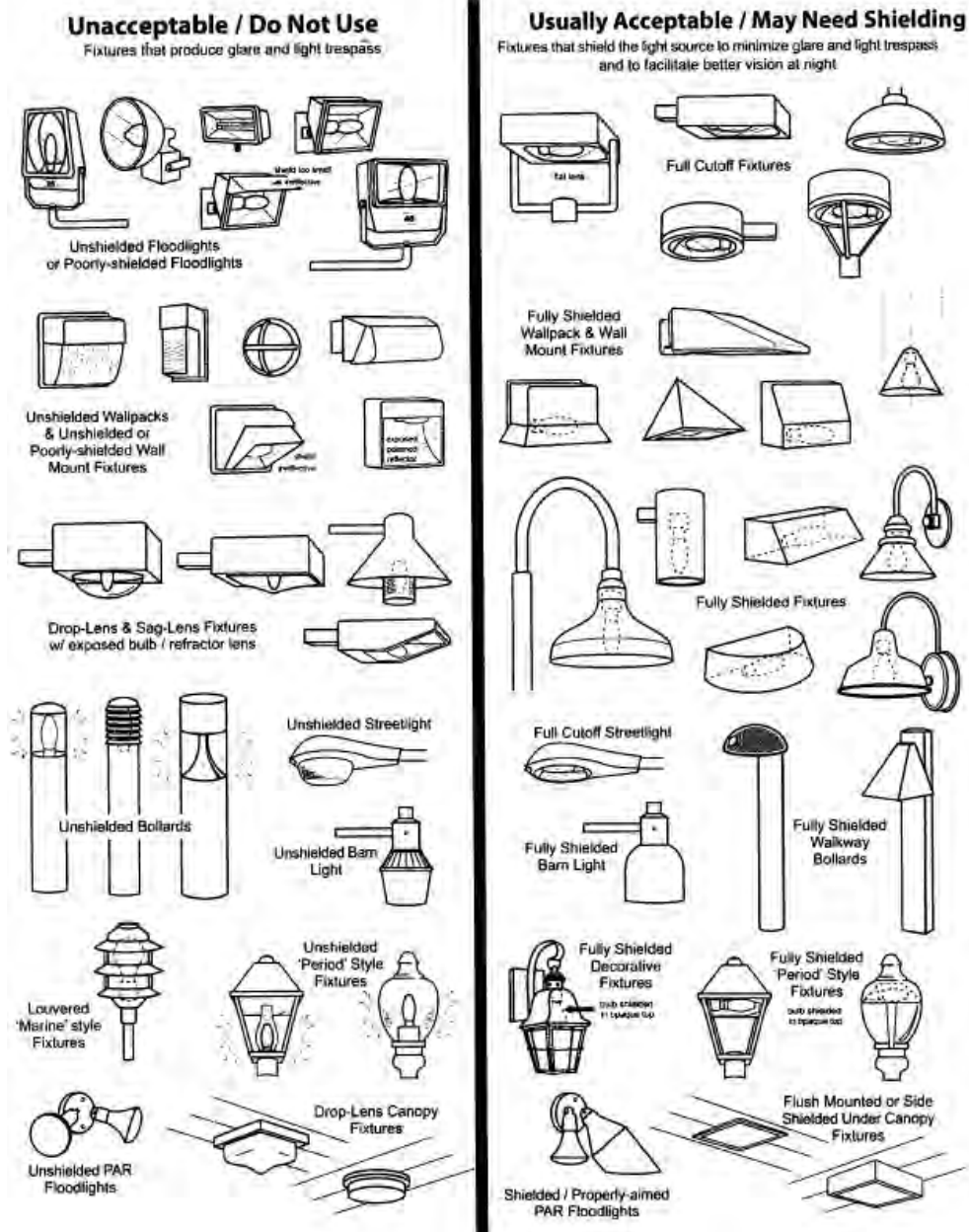
Figure E: The lights on the left are nonconforming. Those on the right can be used in most cases. However, the mounting height and proximity to the property line may cause them to need additional shielding to prevent the luminous elements from being visible from any other property.
