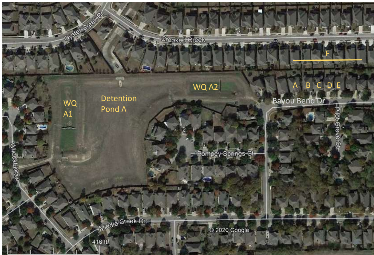
Figure 2. Stormwater facilities and affected homes labeled A-E on Bayou Bend and with line F on Crooked Creek Drive.
