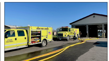
Byron firefighters inspected and tested firehoses and completed the annual firehall maintenance on May 7. Every spring, the firefighters test each firehose by unrolling it and running water through it. The hoses must be able to stand up to high water pressure when they are needed in the field, so the firefighters inspect each hose carefully for any signs of weakness. They also do a deep spring cleaning of the firehall, and they inspect each truck and all equipment to be sure everything is ready to roll when an emergency call comes in.
