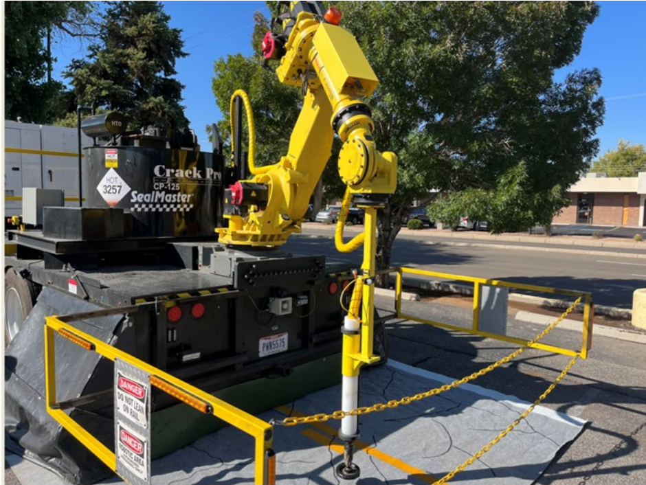
Figure 1. Robotic crack sealing demonstration at a pavement preservation partnership meeting (approximate purchase price of $800,000 or monthly rental of $36,000). 1
