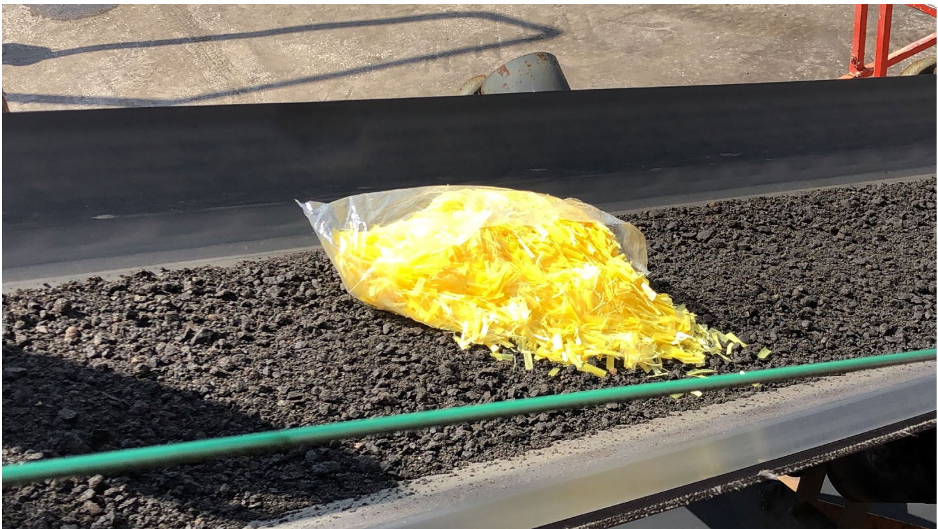
Figure 2. Aramid fibers being introduced into the reclaimed asphalt pavement feeder at an asphalt plant.
