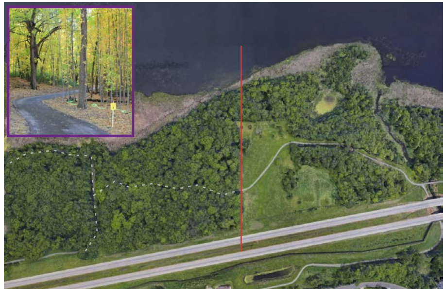
At Rice Marsh Lake, the City of Chanhassen utilized on-site flagging for final trail locations to avoid trees and preserve the canopy of the site. The effects can be seen in the aerial, with the site located trail to the left of the red line, compared with the trail design on the right side, and the obvious cut in the canopy.
