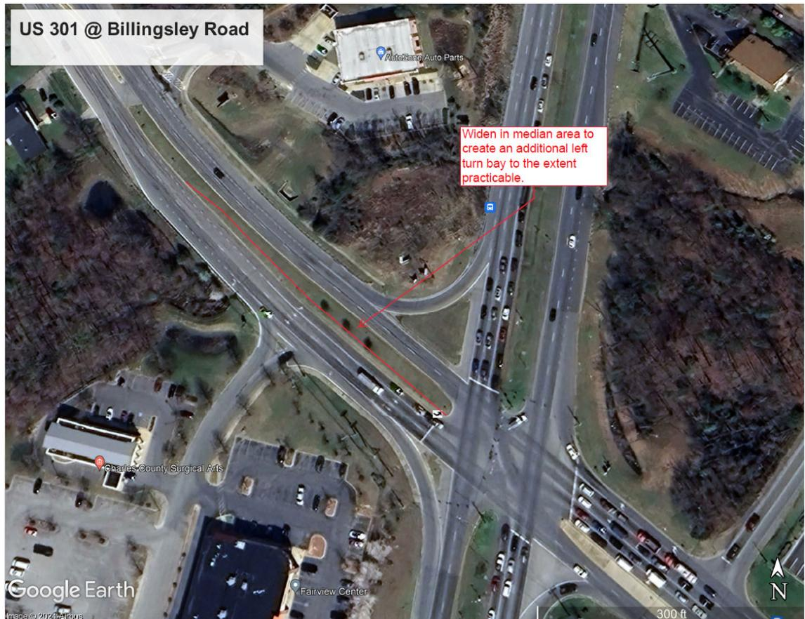
**With this improvement in place, the Synchro/HCM analyses indicate that the v/c ratio will be improved to a level better than background conditions. This improvement will also provide adequate storage area to accommodate total future traffic volumes, including South Park East, South Park West, and Kaiser Permanente. This improvement will over-mitigate the impact of the South Park East project on this intersection. The results of the analyses are shown in the charts below.**
