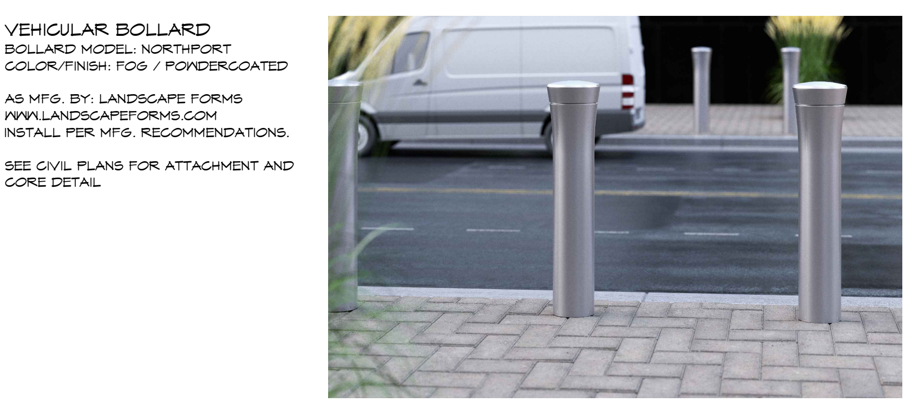
8 DETAIL: VEHICULAR BOLLARD L-5 3/4" x 1'-0"
