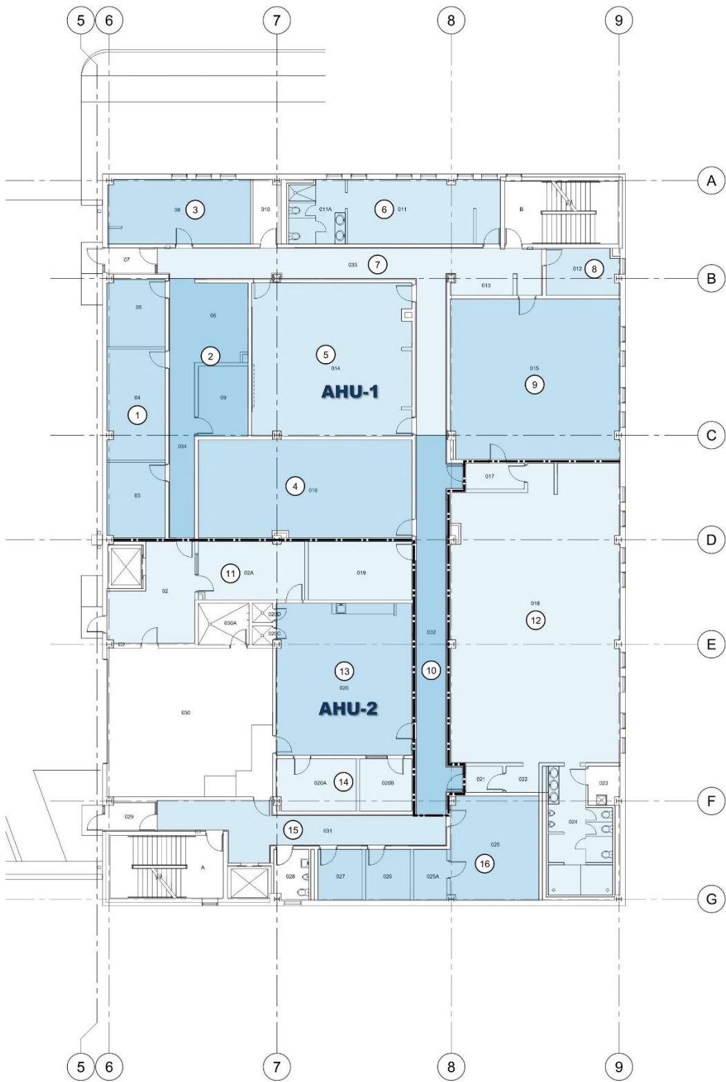
Figure 2 – Lower Level 1 VAV Air Terminal Zones
