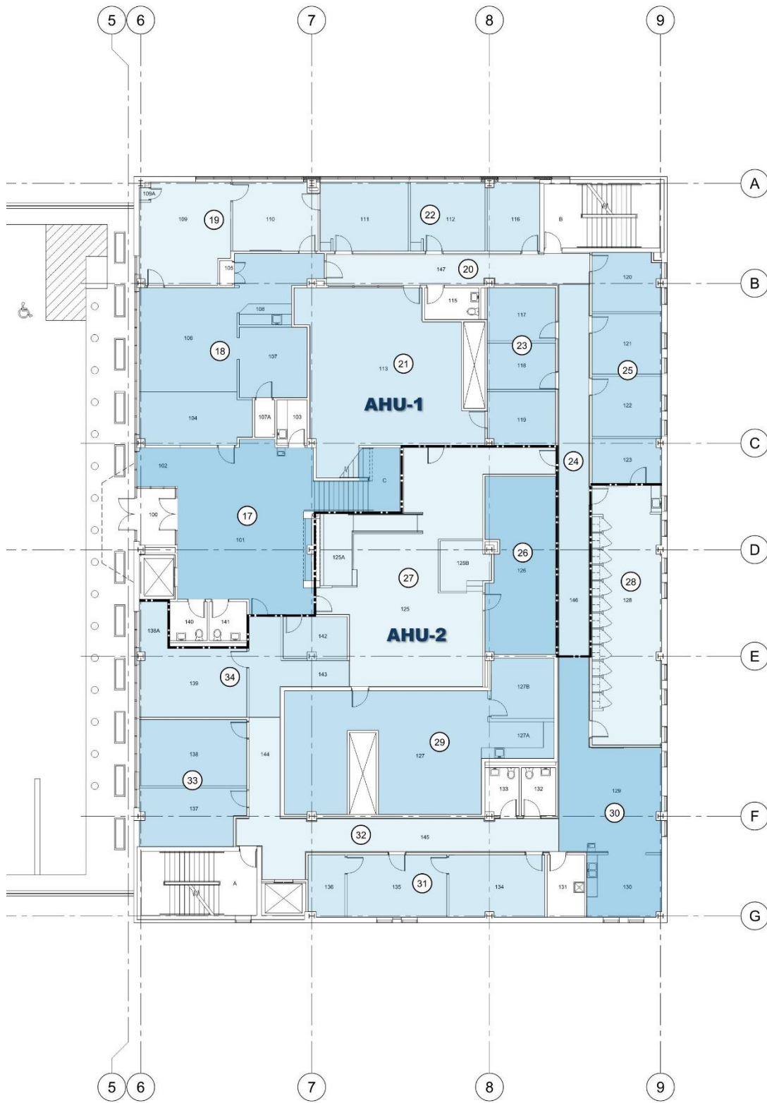
Figure 3 - First Floor VAV Air Terminal Zones
