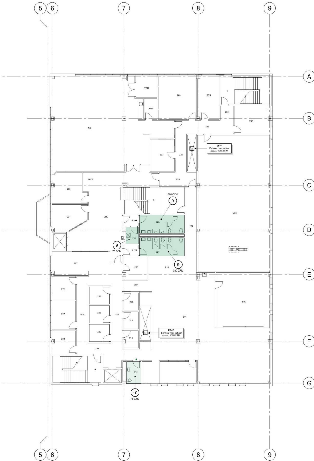
Figure 12 - Second Floor Exhaust Zones
