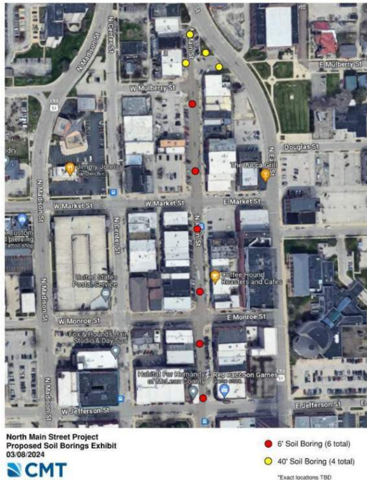
FIGURE 3 – SOIL BORING LOCATIONS
