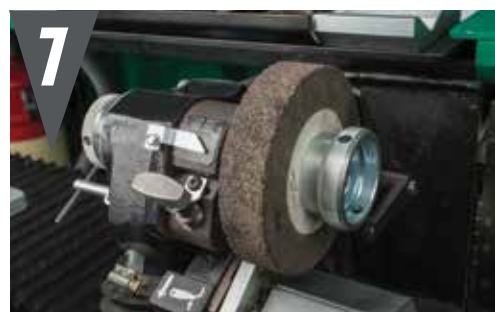
ROBUST GRINDING HEAD & RELIEF ASSEMBLY
