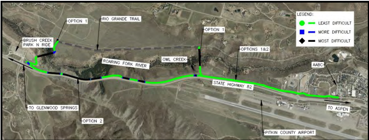
Figure 3-2: Overall Site Map with Alignment Difficulty Levels
