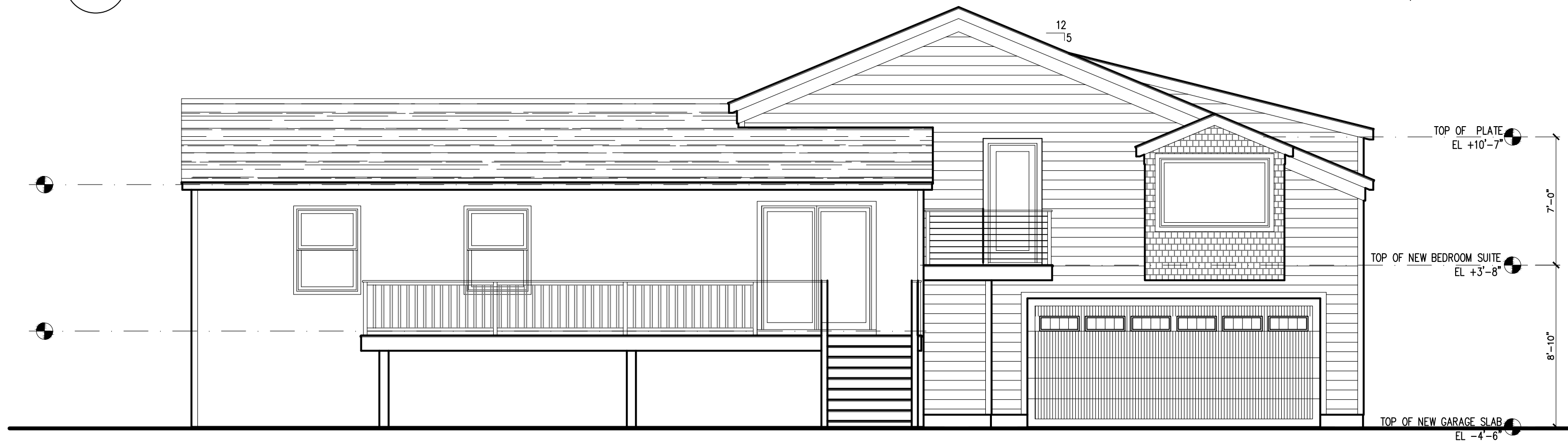
EXISTING SOUTH (REAR) ELEVATION w/ PROPOSED ADDITION
