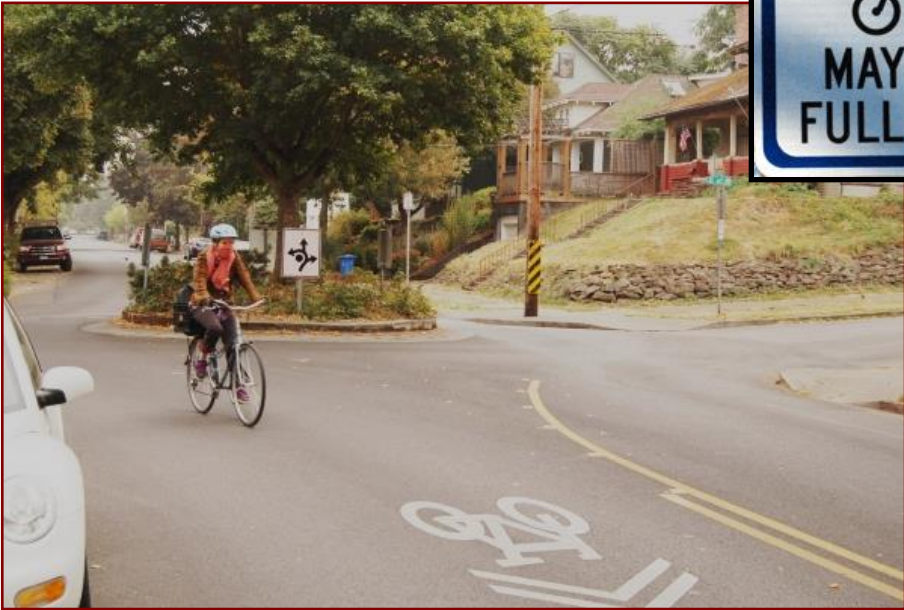
Landscaped intersection circle slows down vehicle speeds, but allows through traffic
