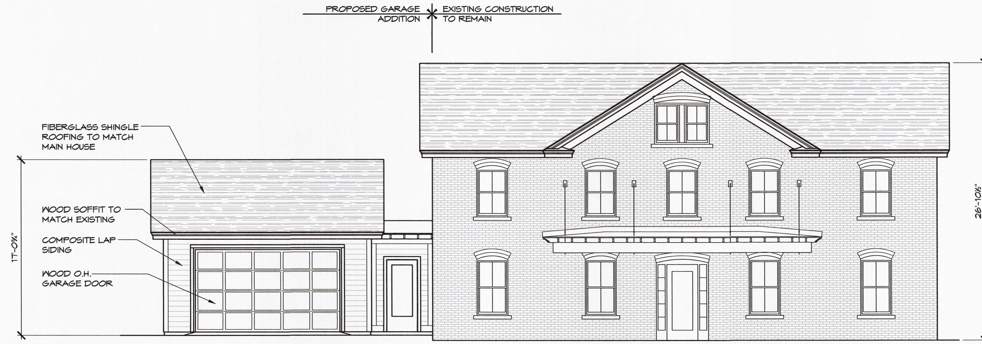
1 EAST ELEVATION C-2 3/16" = 1'-0"
