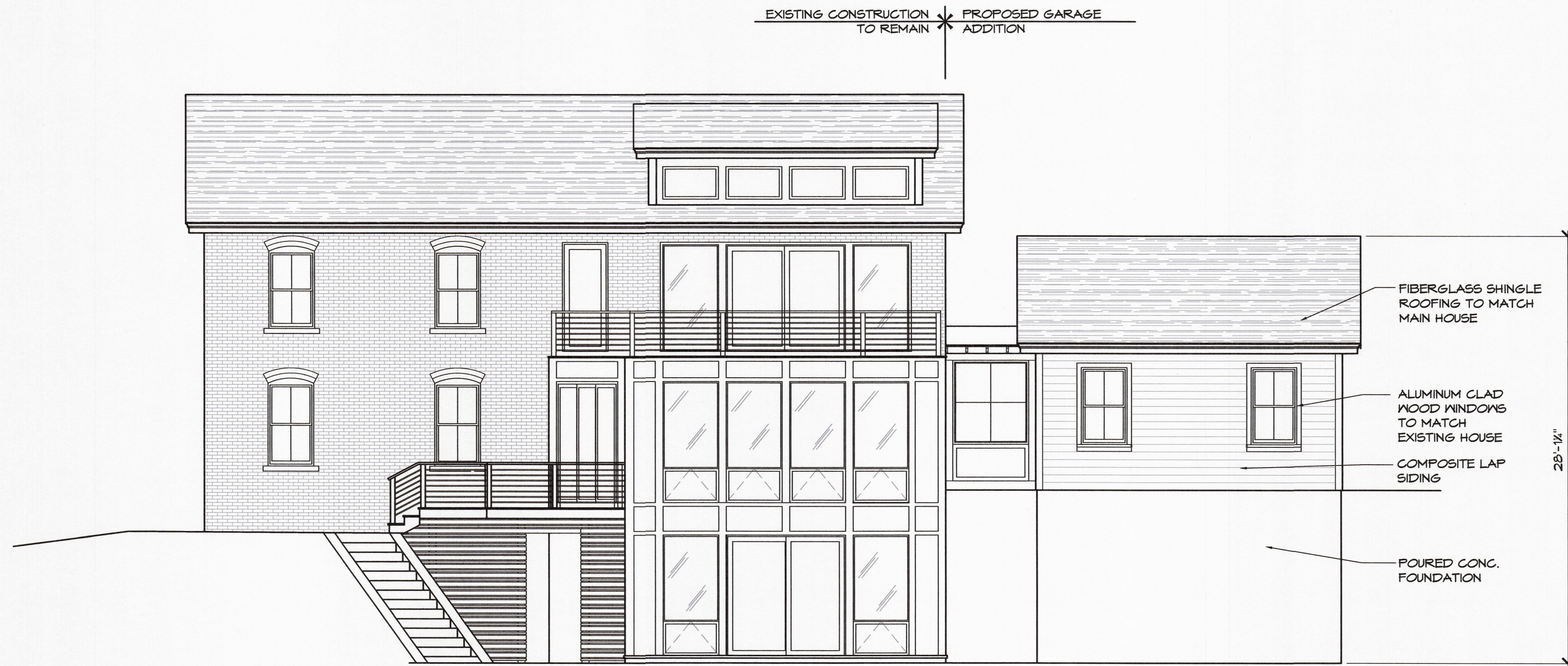
3 WEST ELEVATION C-2 3/16" = 1'-0"
