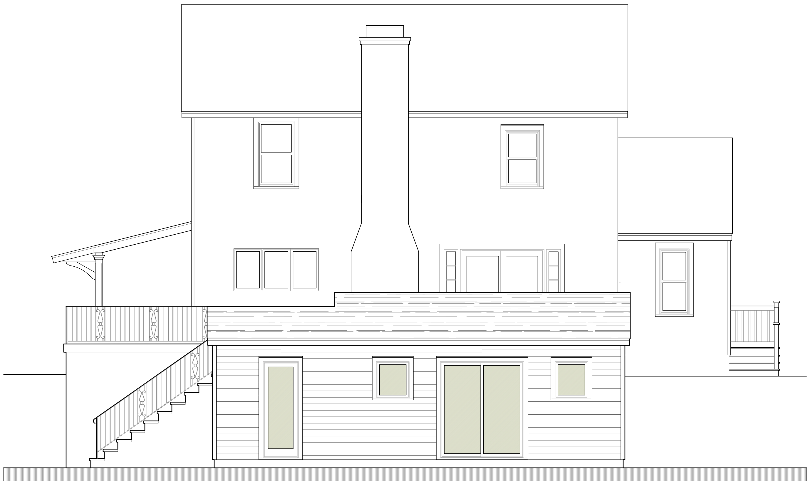
4 PROPOSED WEST ELEVATION 1/4"=1'-0"
