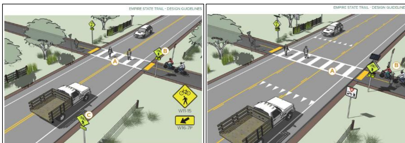
Figure 17: Typical Signage and Striping (left) and RRFB installation (right).
