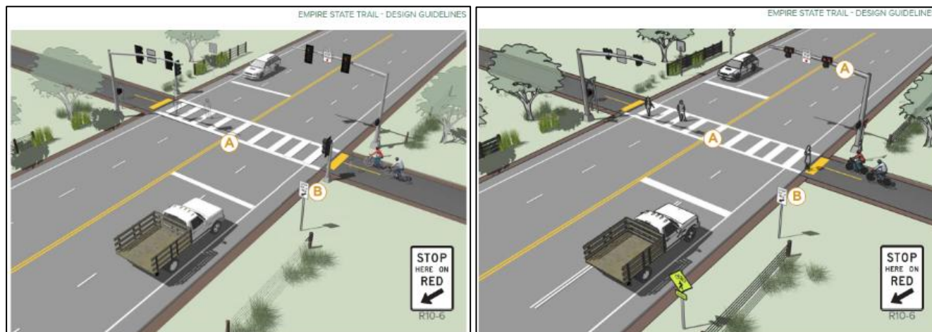
Figure 16: Typical Traffic Signal (left) and HAWK Signal installation (right).
