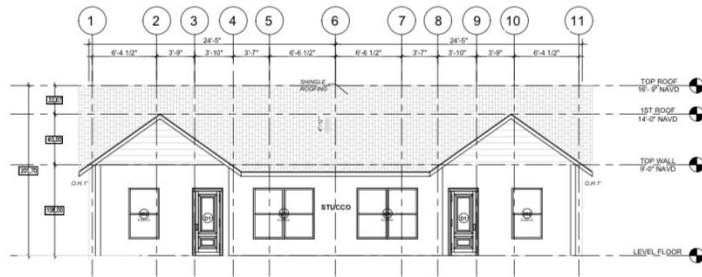
WEST ELEVATION (DIMENSIONED)
