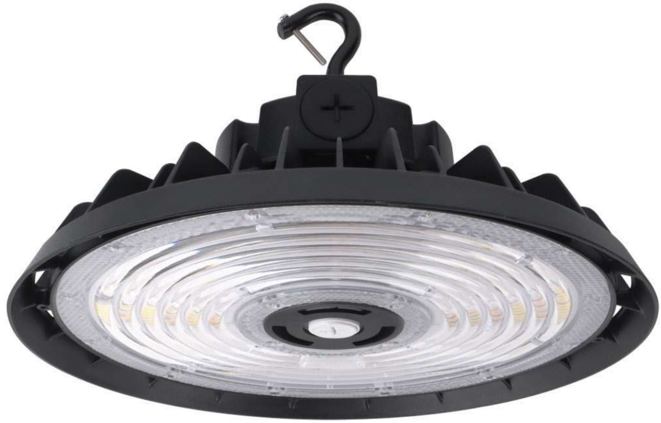
R1 LED Round High Bay 240W, 5000K, 37,463lm, Wattage & CCT Selectable
