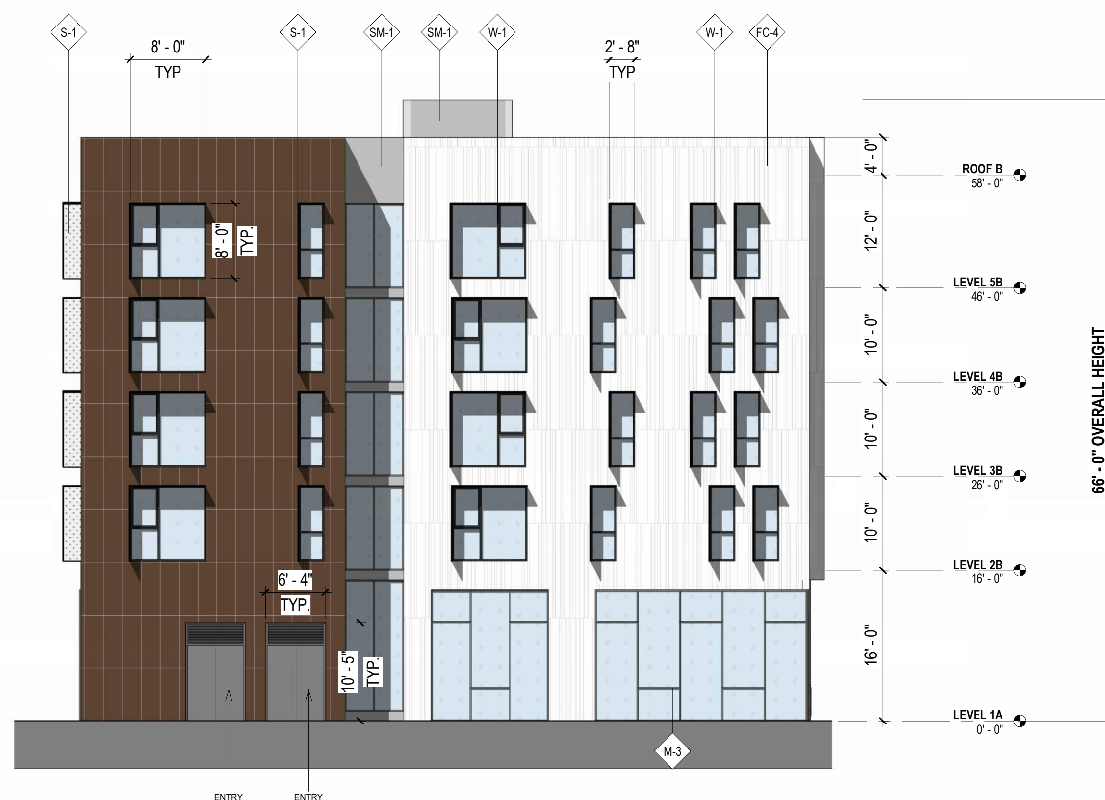
④ BUILDING B ELEVATION - SOUTH 1" = 10'-0"
