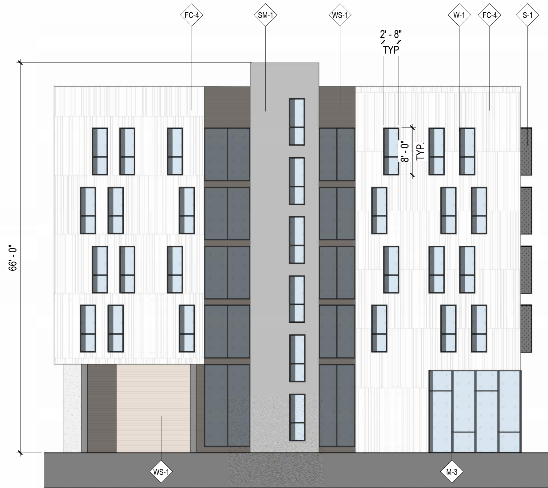
① BUILDING B ELEVATION - NORTH 1" = 10'-0"
