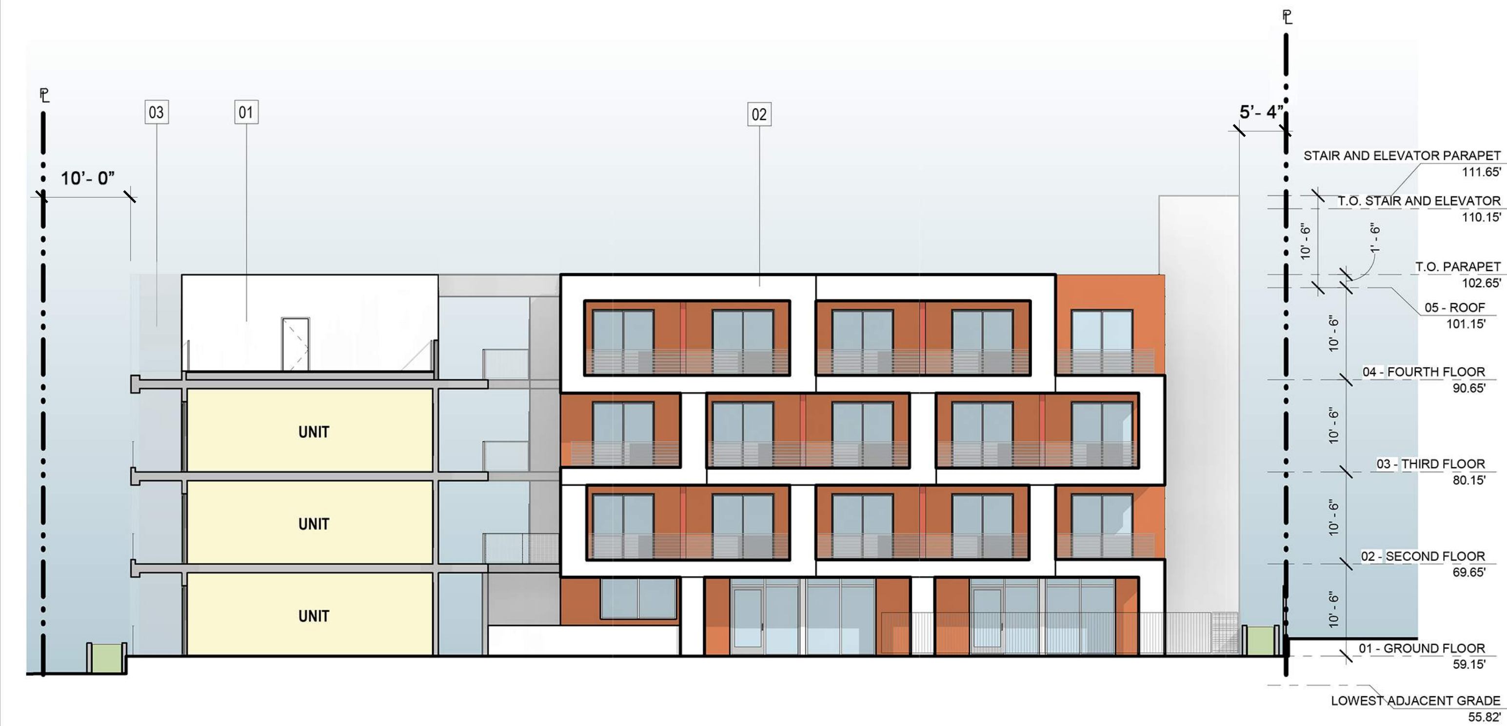
COURTYARD ELEVATION - NORTH SCALE: 3/32" = 1'- 0"
