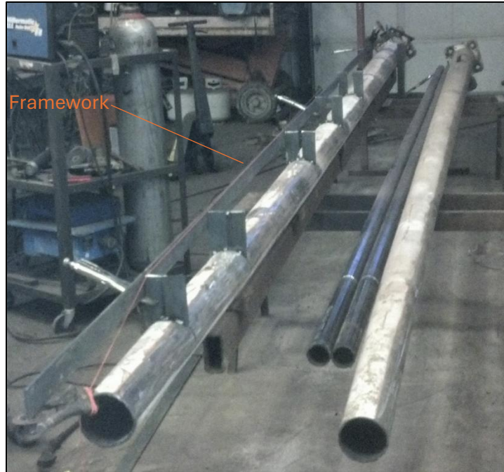
Construction of framework over pole to create airplane wing-like shape
