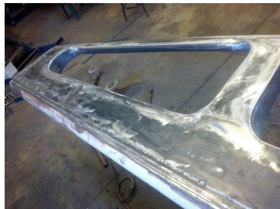
Construction of backstay to create safety pin-like clasp shape at top of each pole
