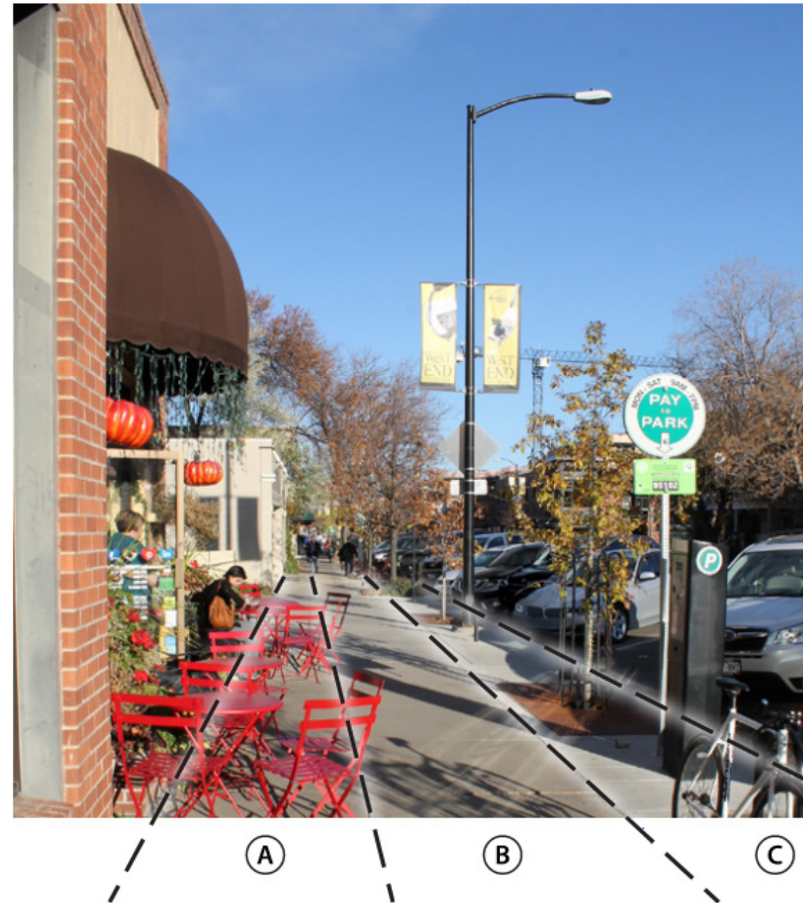
Fig. 36 Diagram of the typical sidewalk zones (Source: City of Boulder)
