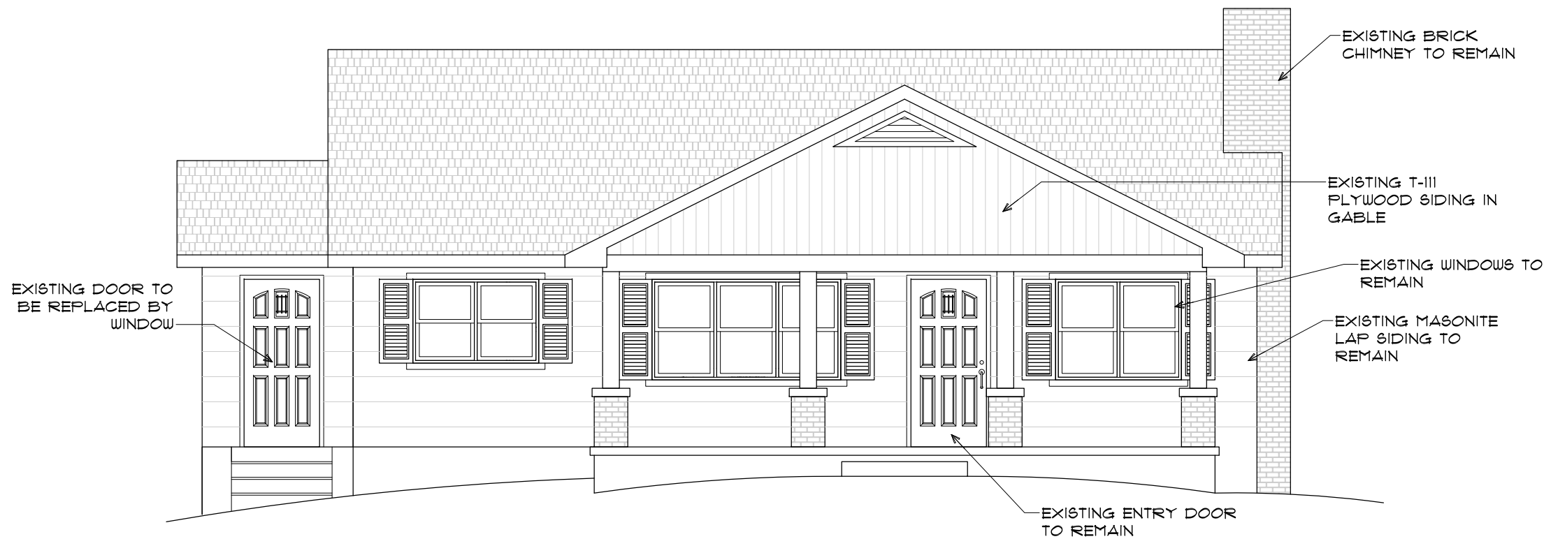
FRONT ELEVATION - EXISTING \frac{3}{16}'' = 1'-0''
