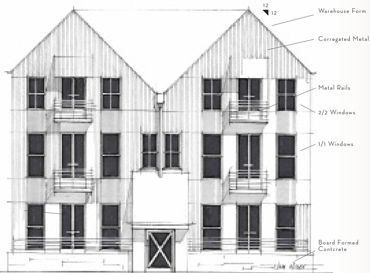
FRONT ELEVATION - INDUSTRIAL VERNACULAR
