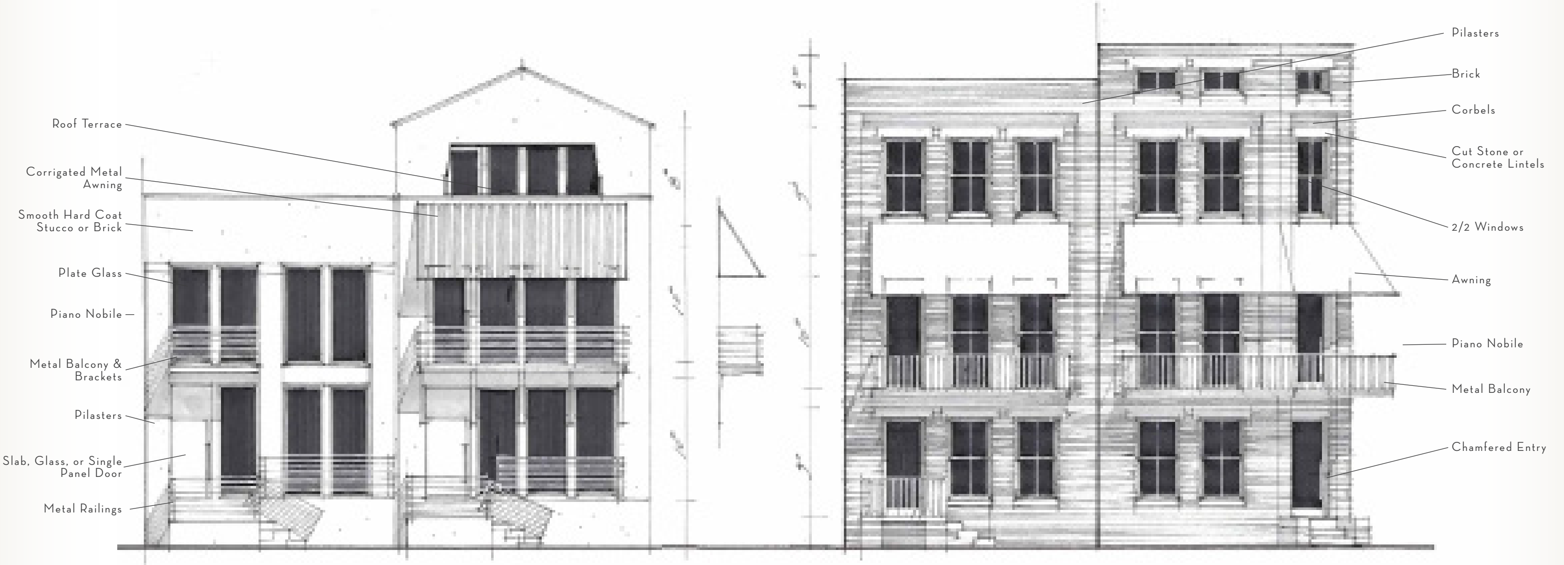
FRONT SIDE ELEVATION - TRANSITIONAL
