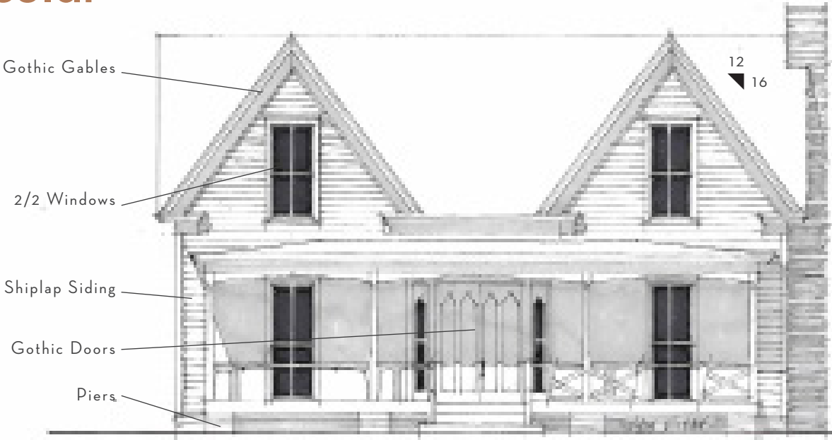
FRONT ELEVATION - VERNACULAR/GOTHIC
