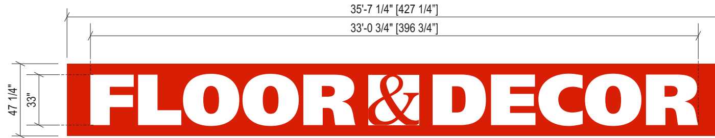
Sign Layout Detail Scale: 3/16" = 1'-0"
