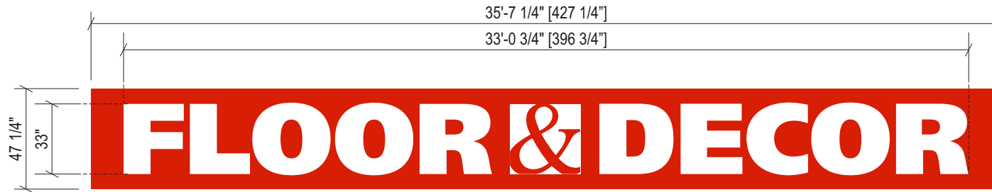
Sign Layout Detail Scale: 3/16" = 1'-0"
