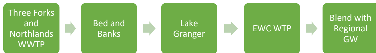
Figure 3.6 IPR to Lake Granger Alternative Process Flow Diagram
