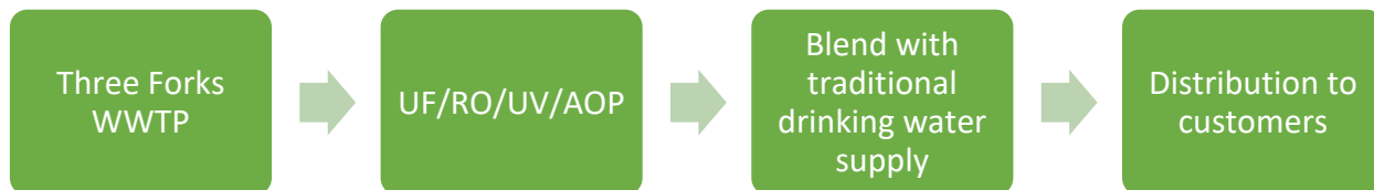
Figure 3.12 DPR at Three Forks WWTP Alternative Process Flow Diagram
