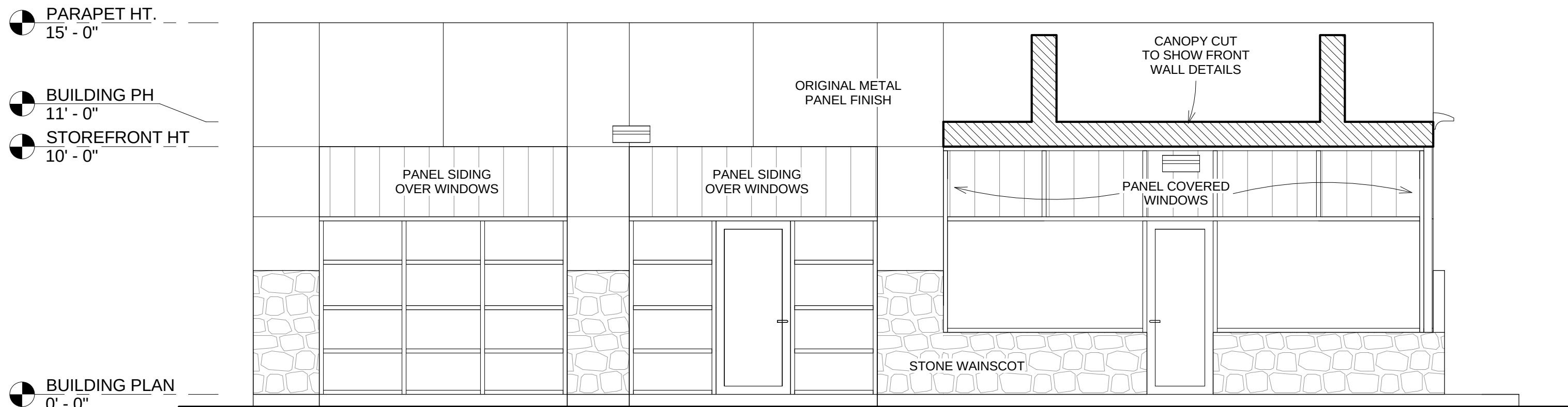
① EXISTING FRONT ELEVATION 1/4" = 1'-0"
