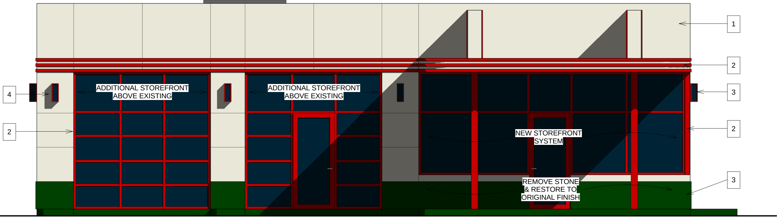
① RENOVATED FRONT ELEVATION 1/4" = 1'-0"
