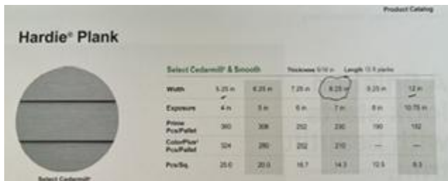
CEMENT FIBER EXTERIOR SIDING 8.25" WIDE WITH 7" EXPOSURE
