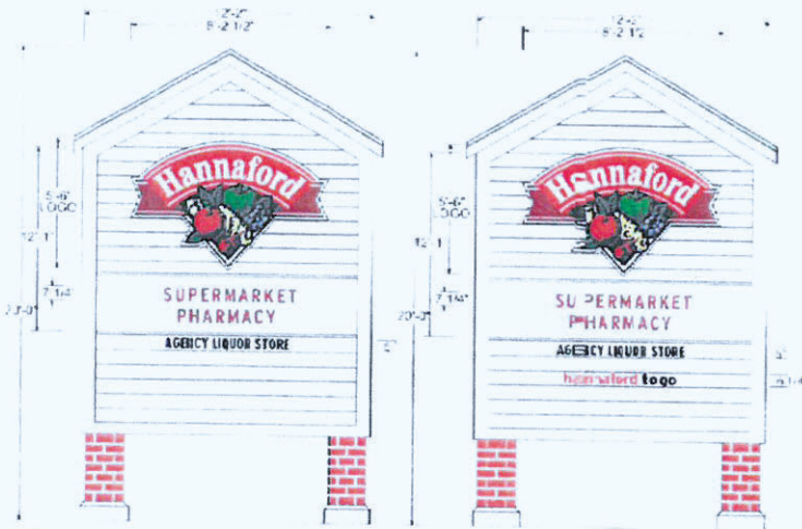
Existing Pylon Elevation Scale: 1/4" = 1'-0" approx.
