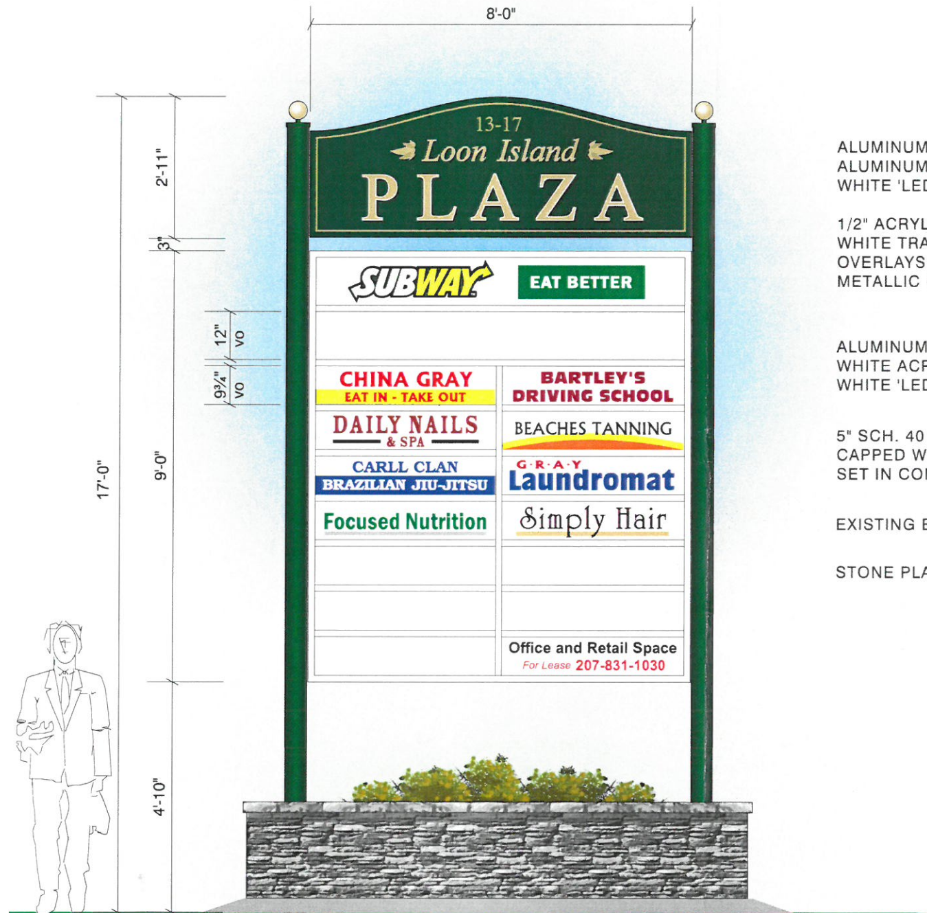
DOUBLE FACE INT. ILLUM. PYLON SCALE: 3/8" = 1'-0" (1) REQUIRED 95.3 SQ FT
