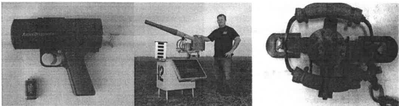
Figure 4. Frightening devices used to disperse ravens include lasers ( left ) and propane cannons. Modified soft-catch traps are also used to live trap the birds ( far right ).
