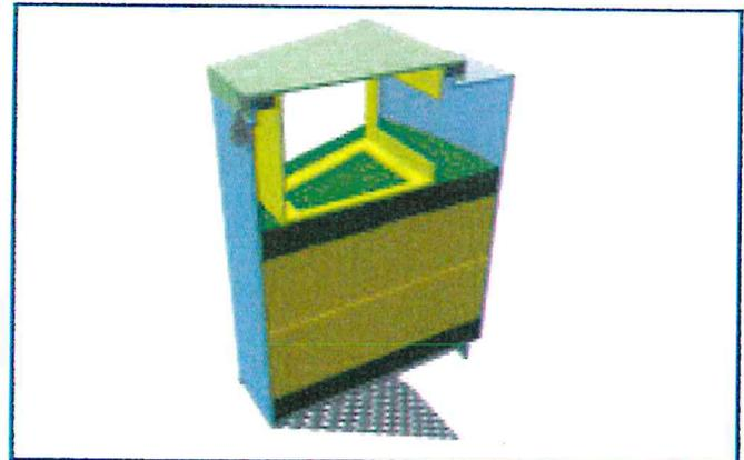
Figure 7: Cut-away view of the Filter Module
