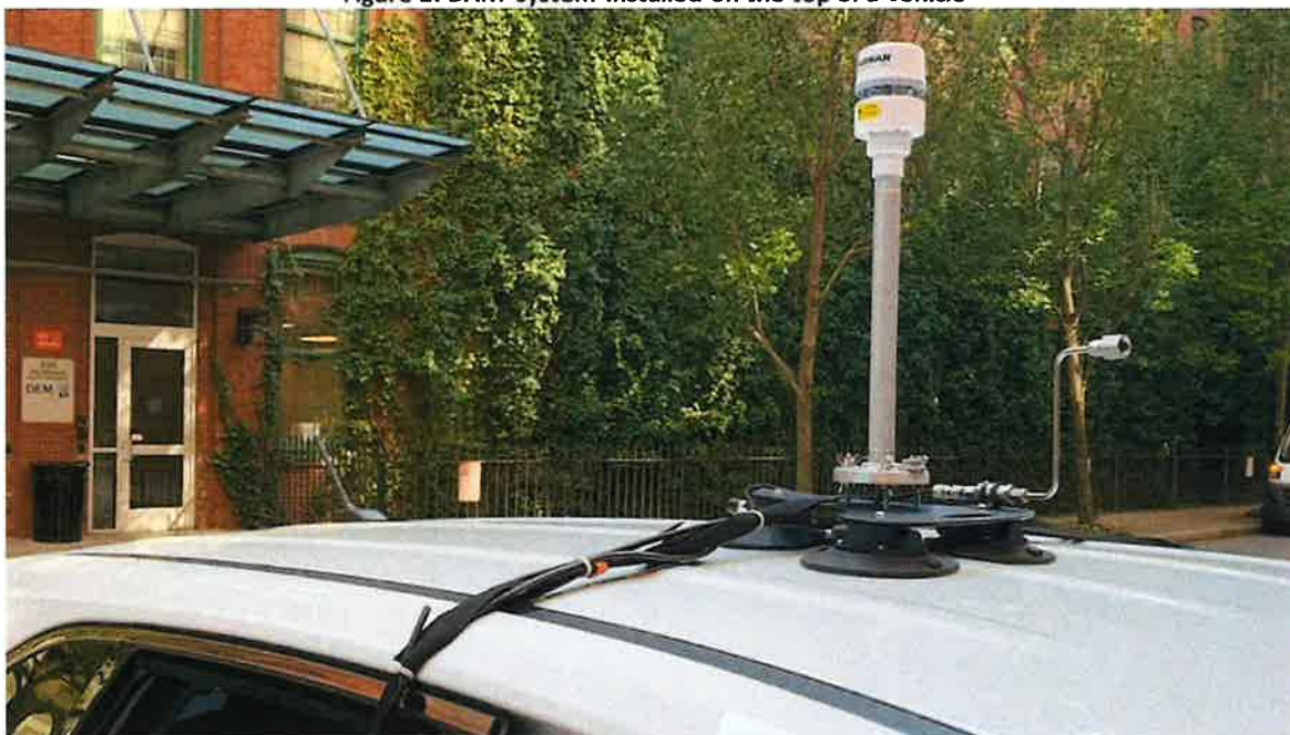
Figure 2: DART system installed on the top of a vehicle
