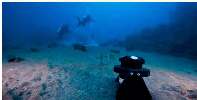
Figure 2. Nortek Signature 1000 Current Meter
