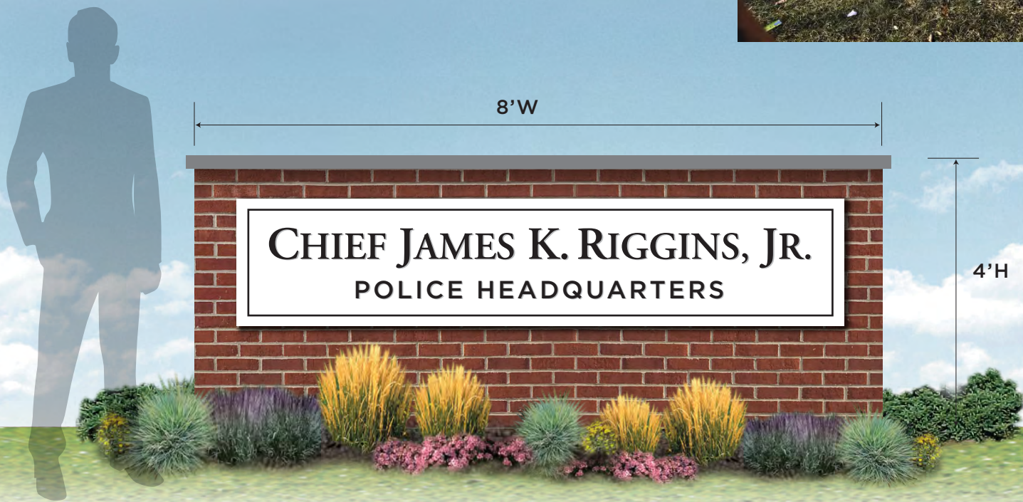
8'W x 4'H x 2'D - brick base with bluestone cap. 1/4" thick painted aluminum lettering - 5"H and 3"H Lettering mounted to a 2" deep fabricated aluminum pan-formed panel.
