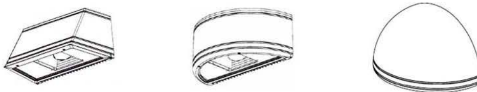
Figure H: Examples of acceptable wall packs.
