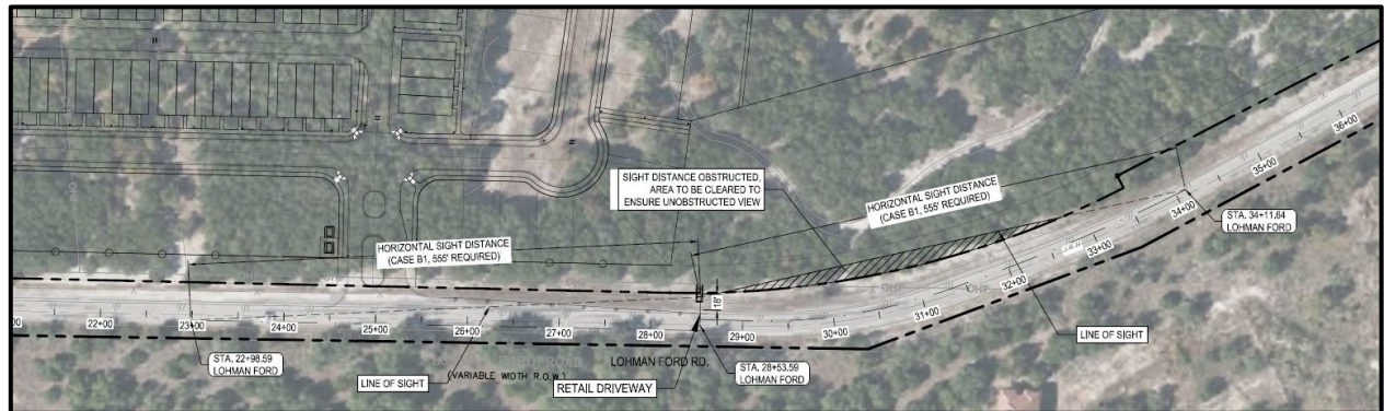
Figure 17 – Retail Driveway #3 Intersection Sight Distance
