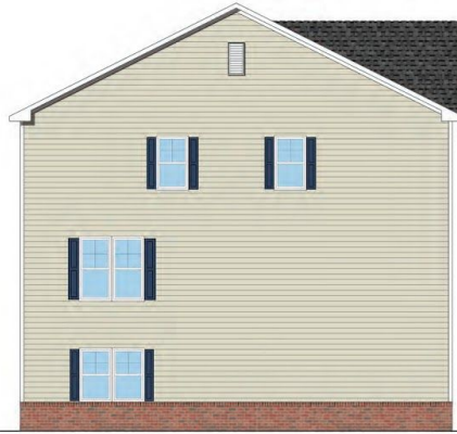
LEFT ELEVATION A :: BRICK WATERTABLE
