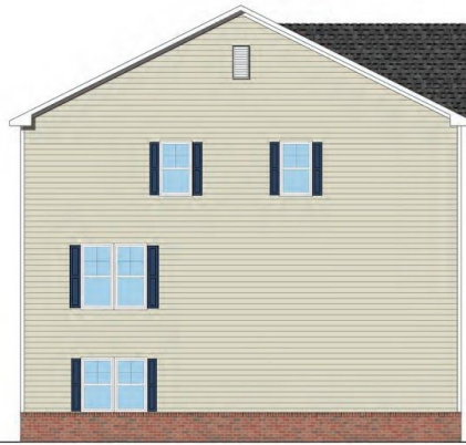
LEFT ELEVATION A :: BRICK WATER TABLE
