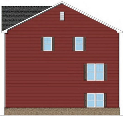
RIGHT ELEVATION A :: BRICK WATER TABLE
