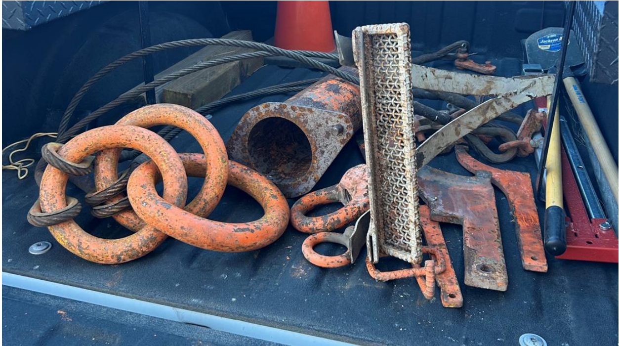
A sampling of equipment removed from the Horsetooth Valve House for lead paint abatement and recoating.
